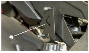
10. Install the rectifier/regulator to the BRKT.,REGULATOR 17 using the NUT,U FLANGE 10.
