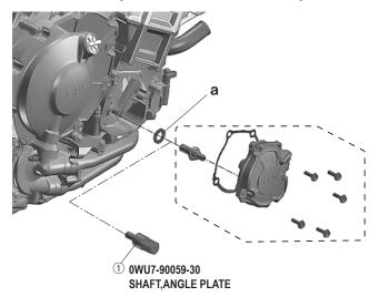
1. Remove the dotted line part (oil pump cover, gasket and bolts) on the right side of the engine and install ①.
