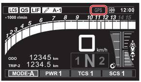
Since the GPS and oil-pressure warning icons are at the same location, the GPS icon does not light up when the the oil-pressure warning icon lights up (such as engine stop).
