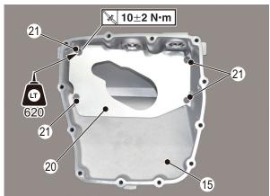
8. Attach (15) PAN,OIL to the engine by using (16)BOLT,BUTTON HEAD.
