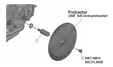
Attach the prepared protractor using ②.
