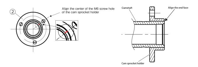
4.Assemble the kit cam sprocket in the position where the mark made in step 1. and the "B3L" mark are diagonal.
