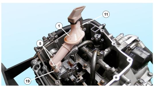
Fix (1) STRAINER HSG.ASSY., 11 PIPE, DELIVERY 1 and (23)BRKT.,STRAINER
