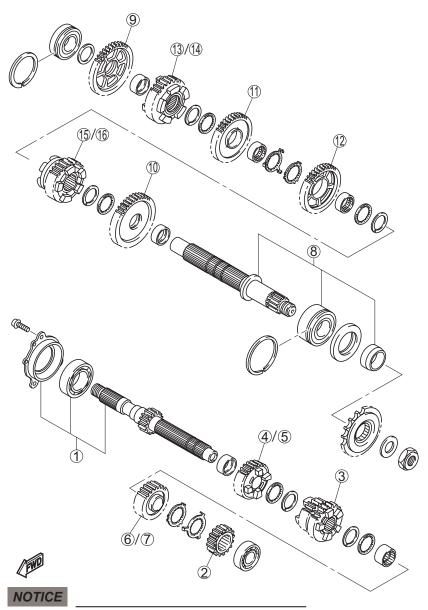
This set contains modified gear ratios and docks compared with the STD gearbox.
