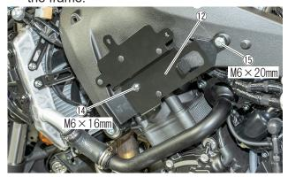
5. Install the ECU and BRKT., UPPER (1) using the BOLT, FLG (6) to the BRKT., UNDER(2).
