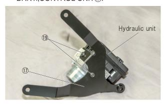
7. Install the BRKT., CONTROL UNIT® using the STD Bolt and collar, BOLT, HEX. SOCKET HEAD® to the vehicle.
