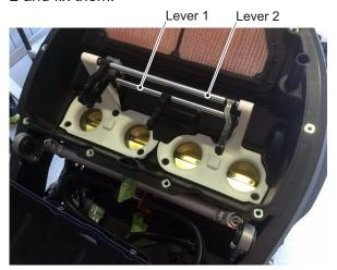
2. Assembling the secondary funnel Install the secondary funnel to the lever 1 and 2. Then, fit the STD bushes to the lever assembling positions. (5 locations)
